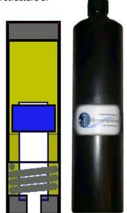
Another feature of your hydrophone allows full protection of the sensitive element, located in the window behind the Oceanphonics label, not at the bottom where it could typically be damaged by rocks on the ocean floor or by being dropped on concrete.
