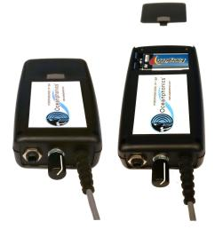
Install the battery pack into the enclosure re-insert the cover.
